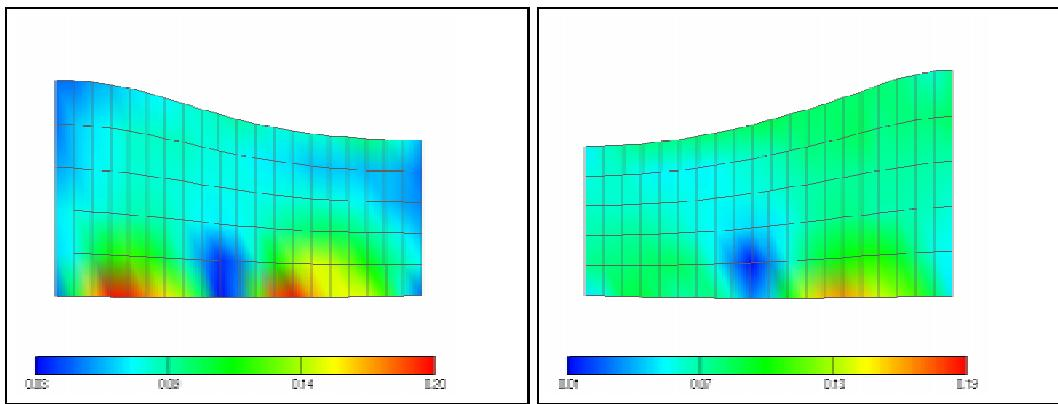
Figure 2: Forced vibrations of a partially filled tank with flexible bottom. Free surface profiles and magnitude of the velocity at  $4.0$  and  $4.6$  sec.
