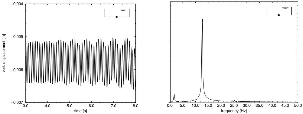
Figure 3: Forced vibrations of a partially filled container with flexible bottom. Motion of the bottom centerpoint and Frequency spectrum. The span  $t = 3.0 - 8.0$  s is representative of the entire simulation.
