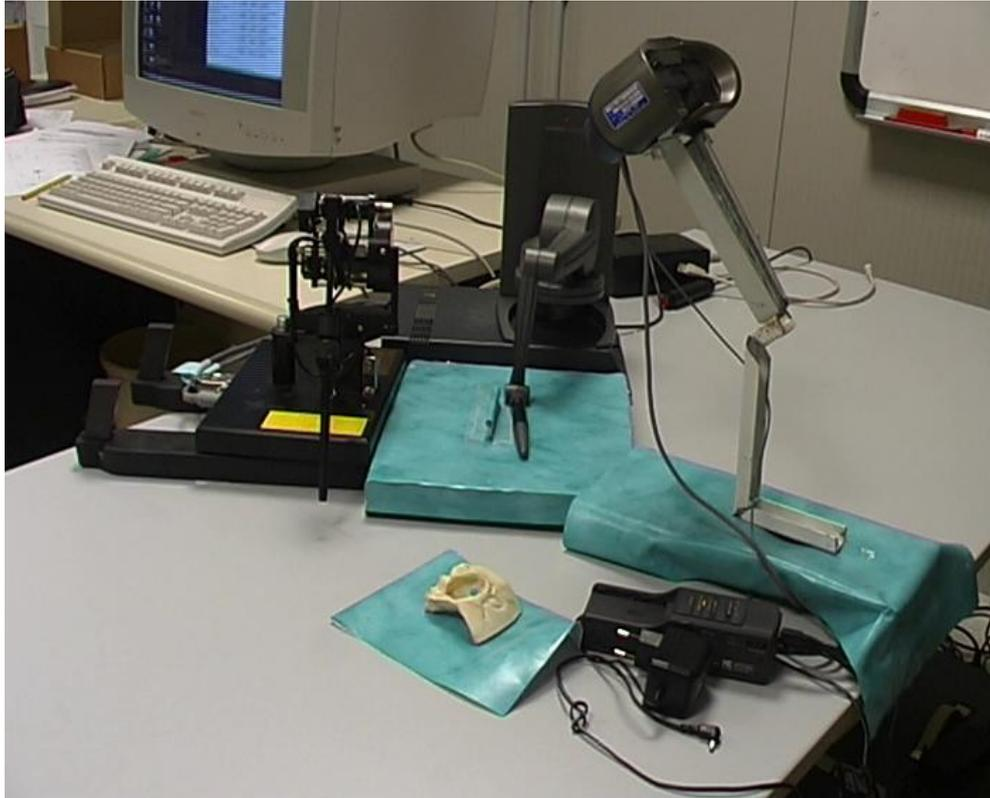
Figure 3.1: The current Ierapsi surgical simulator set-up. Note the Phantom Desktop haptic device for the dominant hand; the Phantom 1.0 haptic device for the non-dominant hand and the n-vision VB30 binocular display. The system is driven by, not shown in figure, a single-processor PIII/600 MHz with 256 MB PC100 RAM (haptic loop) and a dual-processor PIII/600 MHz with 512 MB PC800 RAM and a NVIDIA GeForce 2 GTS.
