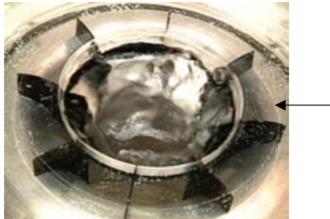
FIG. 5. The free surface in the co-axial target experiment with the anti-swirl device.
