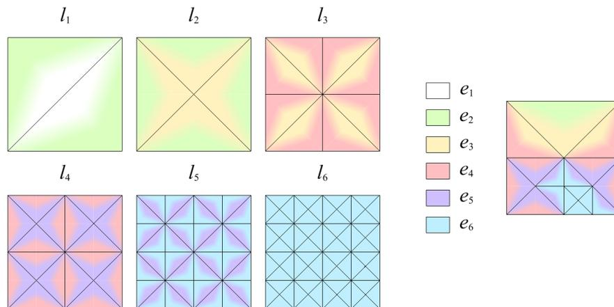
**Fig. 2. An example of a BDAM:** each triangle represents a terrain patch composed by many triangles. Colors correspond to different errors; the blending of the color inside each triangle corresponds to the smooth error variation inside each patch.
