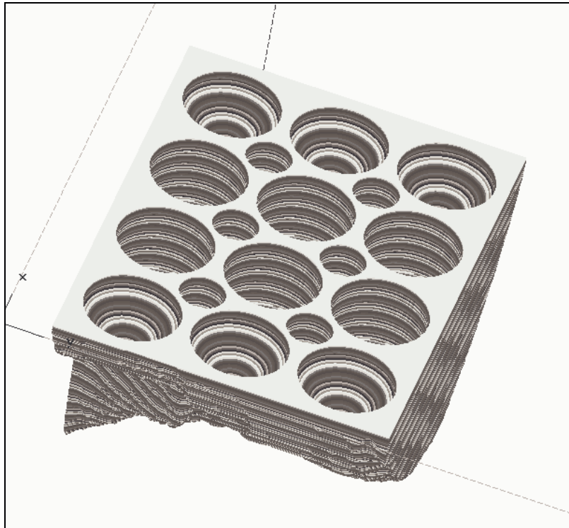
Fig.5. Bottom of the sample: the holes have been made to optimize material use and printing time.
