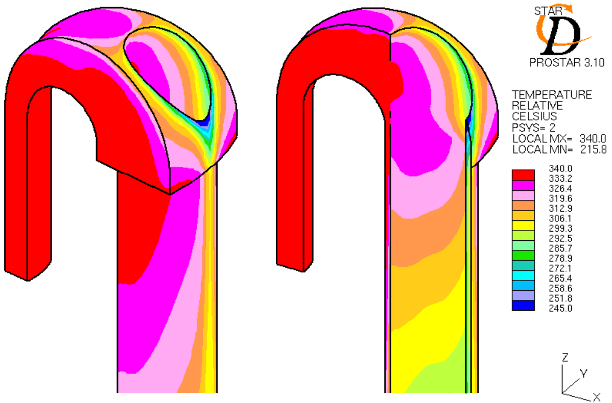
Figure 23 - Case s3: PbBi temperature field in the top part of the target; full and half model. Data are averaged on model vertices.
