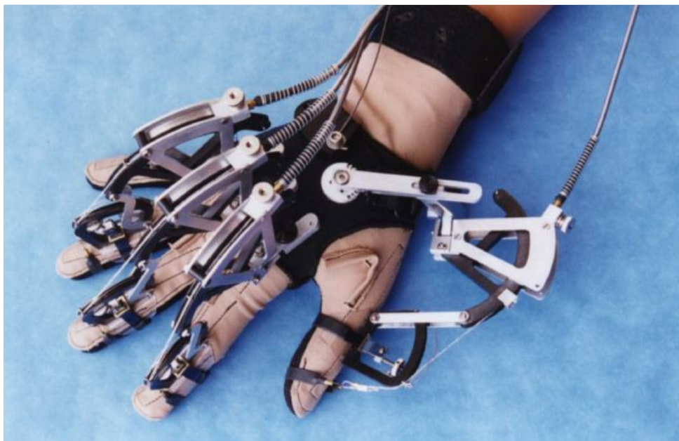
Figure 5.1.: CyberGrasp glove: With the CyberGrasp force feedback system, users are able to feel the size and shape of computer-generated 3D objects. Photo from Immersion Corporation site http://www.immersion.com
