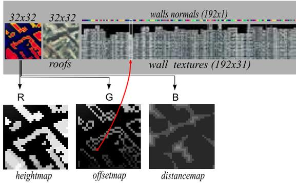
**Figure 2:** In the upper part a the  $256 \times 32$  texture coding a  $32:192$  BlockMap is shown. The bottom part shows the three channels of the first quad, named geometry, of the BlockMap. The red arrow illustrate the texture 2 fetches executed if a vertical wall is hit.
