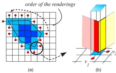
**Figure 4:** Construction of a BlockMap: (a) Height map with boundary texels rendered in cyan. The red dots correspond to the locations from which the renderings are done. (b) Example of a boundary texel with two exposed sides, the two side renderings are averaged together.
