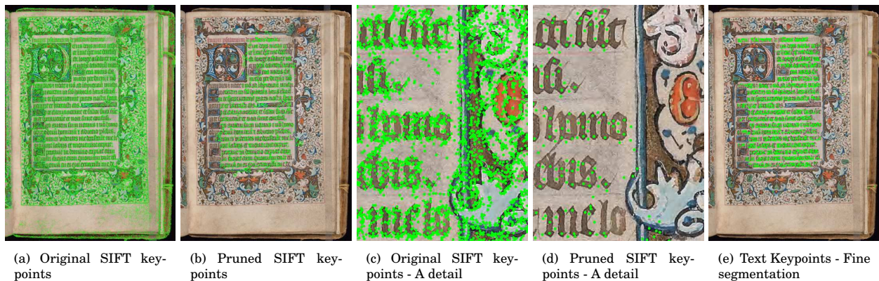
Fig. 6. Text features. The green dots represent the position of keypoints in the image: a) original keypoints; b) pruned keypoints that lie in the coarsely segmented region, and have a scale compatible with the size of the text height; c) and d) zoomed regions showing the pruning operation. Finally we show the refined text feature classification in e). Manuscript images courtesy of the Yale University [BeineckeMS310].
