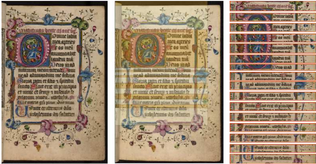
Fig. 13. Our technique vs T-pen. A comparison between the proposed automatic text line segmentation method and the one employed in T-pen [T-pen 2013], a broadly used web service for computer assisted transcription. From left to right: a page from a manuscript, line segmentation of T-pen, our line extraction. Manuscript images courtesy of the Oxford University[BodleianMSBodleian113 ].
