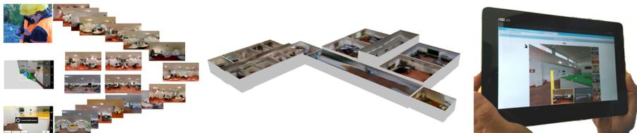
**Fig. 1.** Our method at a glance: from a set of panoramic photos (left) our system computes a textured 3D model of the indoor boundaries (center) which can be explored with a low-degree-of-freedom web application (right).
