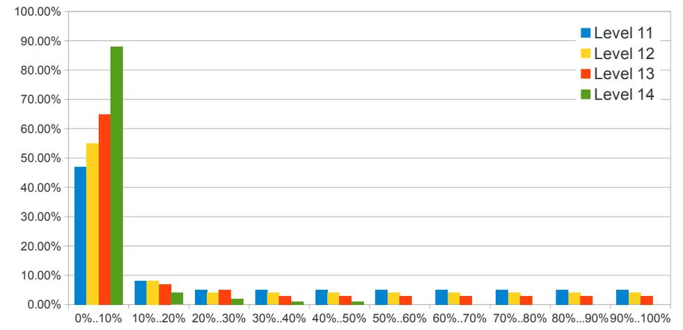
**Figure 5.** Histograms of the references to nodes in the Powerplant dataset voxelized at  $64K^3$  resolution, with nodes sorted by reference counts. As we can see, the distribution is highly skewed, and the most popular 10% of the nodes account for most of the references.
