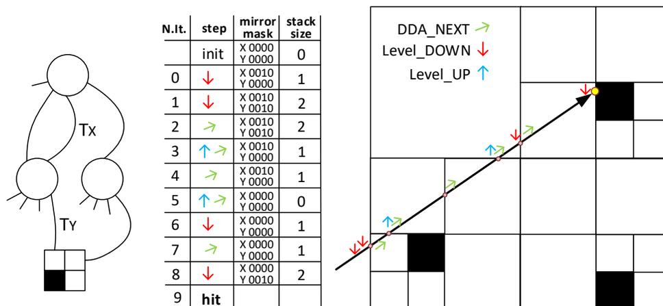
**Figure 7.** Example of traversal. At left, the example tree, with mirror tags on some pointers. Center, the table of iteration with main actions, current node mirror mask and stack size. At right, a representation of same traversal, with the ray passing through the structure up to find the first intersection.
