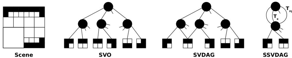
**Figure 2.** Example 2D scene transformed into different structures, with children ordered left to right, top to bottom. The Sparse Voxel Octree (SVO) contains 10 nodes. The Sparse Voxel Directed Acyclic Graph (SVDAG) finds one match and then shares a node, meaning 9 nodes. The presented Symmetry-aware Sparse Voxel Directed Acyclic Graph (SSVDAG) finds reflective matches in two last levels, and reduces the structure to 4 nodes.
