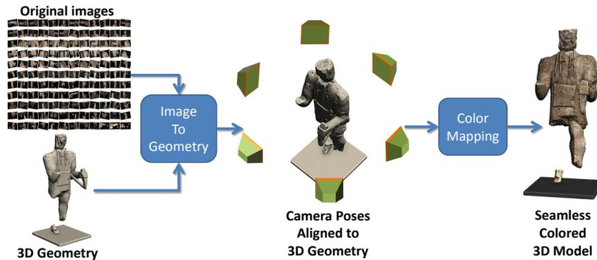
**Fig. 1 Pipeline overview.** The input data is a 3D geometry and a set of photos of the real object. First, an image-to-geometry alignment step registers the images to the 3D model, by producing a set of corresponding camera poses. By exploiting the resulting link between 3D points and pixels, a color mapping procedure produces a seamless color signal across the surface.
