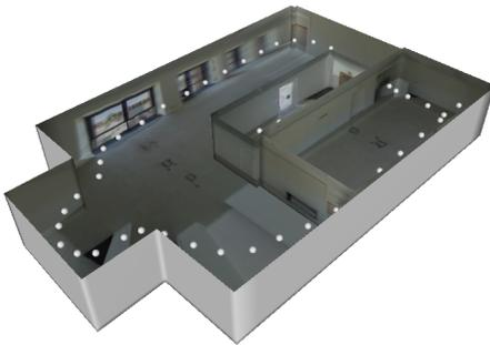
**Figure 6: Office complex of 300 square meters reconstructed from 40 images (grey spheres in the illustration show user poses), acquired by a Ricoh Theta S camera driven by an HTC One M8 smartphone. This scene includes an open space and two big rooms embedded into the main space, resulting in a complex topology with several hidden points-of-view.**
