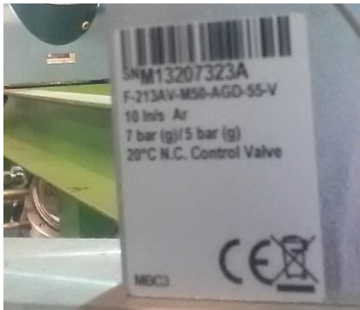
Annex B Fig. 4: Argon mass flow controller identification plate
