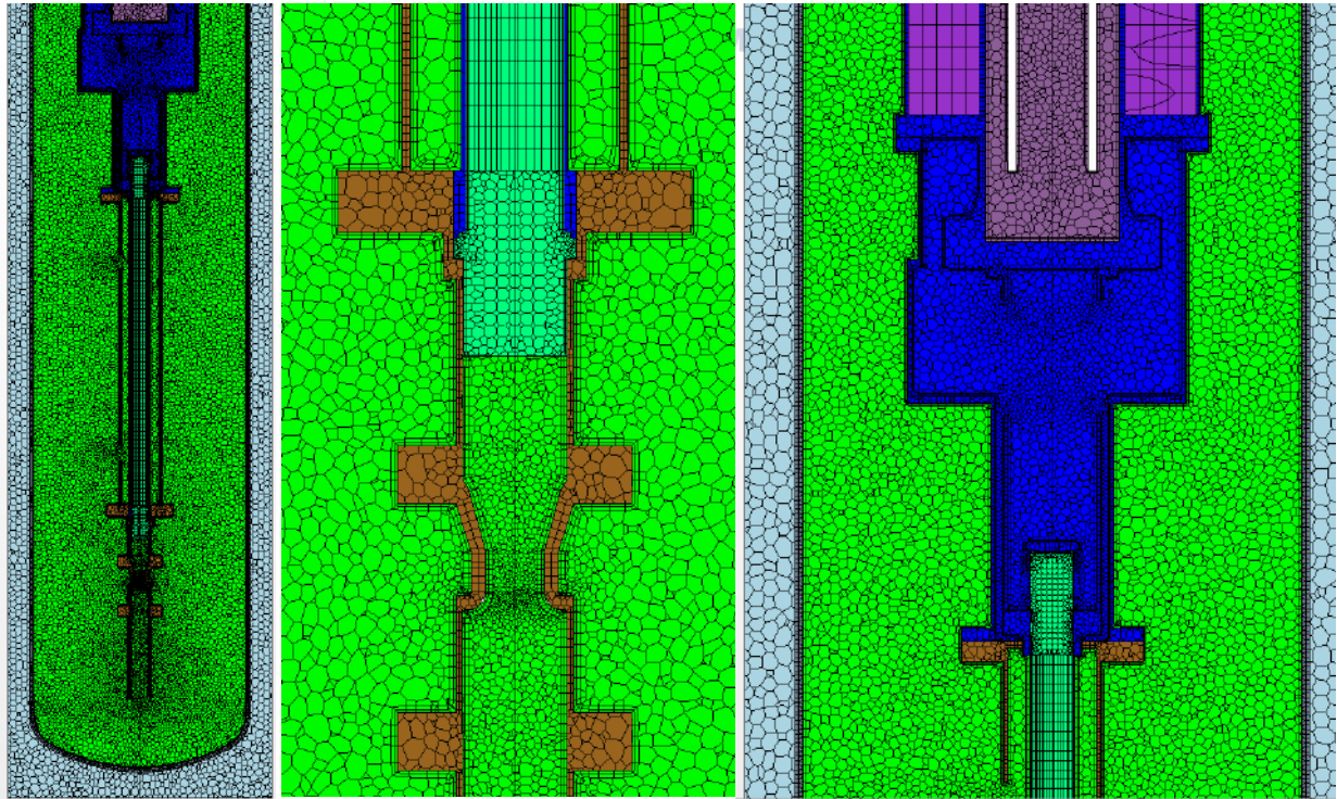
Figure 281: Mesh vertical sections across the pin simulator channel
