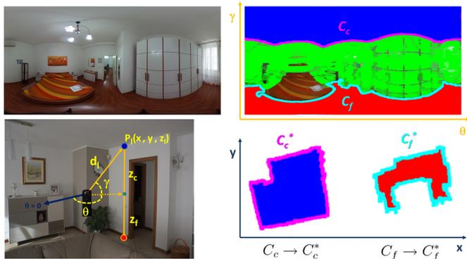
**Fig. 3. Image analysis and Cartesian mapping.** Each image (top left) is automatically labeled as *ceiling*, *wall*, *floor*, *unknown*, with the goal of finding contours between the labeled zones (top right). Contours are transformed through a mapping function from spherical to Cartesian space (bottom right).
