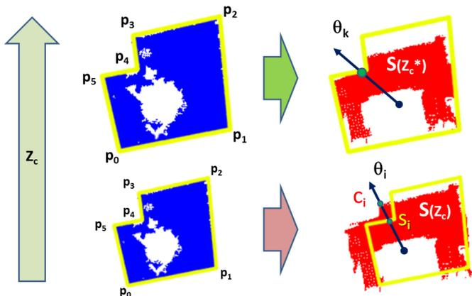
**Fig. 4. Contours scaling and matching.** To recover the 2D room shape from the transformed contours  $C_c^*$  (up-to-scale) and  $C_f^*$  (target metric scale) of eq. 2, we fit the polygon  $S(z_c)$  (yellow - polygonal approximation of  $C_c^*$ ) on  $C_f^*$ , varying  $z_c$  (red arrow), until the best scaling (green arrow) has been found.
