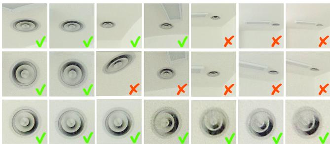
Fig. 10. Spherical vs Cubemaps vs Rectified. We compare object recognition of an almost circular shape on the original equirectangular images (first row), using cubemaps (second row) and with our rectified images (third row). Successfully retrievals are marked with a green check.
