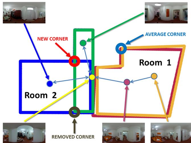
**Fig. 5. Multiple poses merging.** Single reconstruction are merged exploiting multi-view alignment between overlapping images. More than one reconstruction per room are exploited to refine the same room shape (Room1, orange and magenta), or joined to cover hidden corners (Room2 is fully covered by the green and blue reconstruction). Intermediate poses can connect different rooms (yellow).
