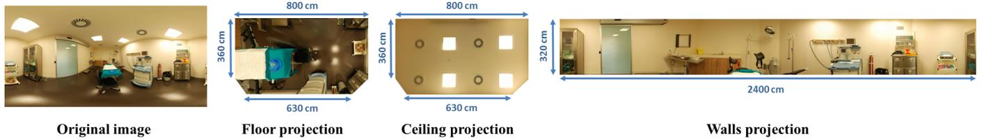
Fig. 6. Rectification. For each original equirectangular image we generate three bi-dimensional images in uniform metric dimensions: floor, ceiling and walls images. The ceiling projection shows how two of the four air ducts, practically unrecognizable in the original image, are instead clearly highlighted in the rectified image.
