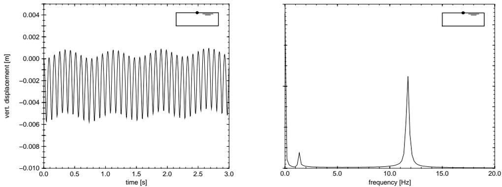
Figure 1: Vibration of a partially filled container with flexible bottom. Vertical displacement of the free surface centerpoint.
