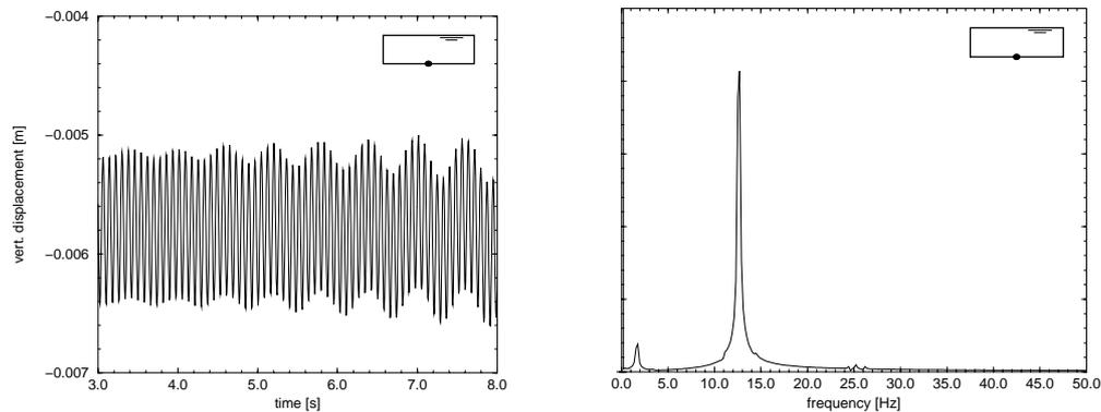
Figure 3: Forced vibrations of a partially filled container with flexible bottom. Motion of the bottom centerpoint and Frequency spectrum. The span  $t = 3.0 - 8.0$  s is representative of the entire simulation.
