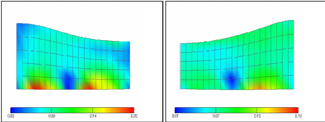
Figure 2: Forced vibrations of a partially filled tank with flexible bottom. Free surface profiles and magnitude of the velocity at 4.0 and 4.6 sec.
