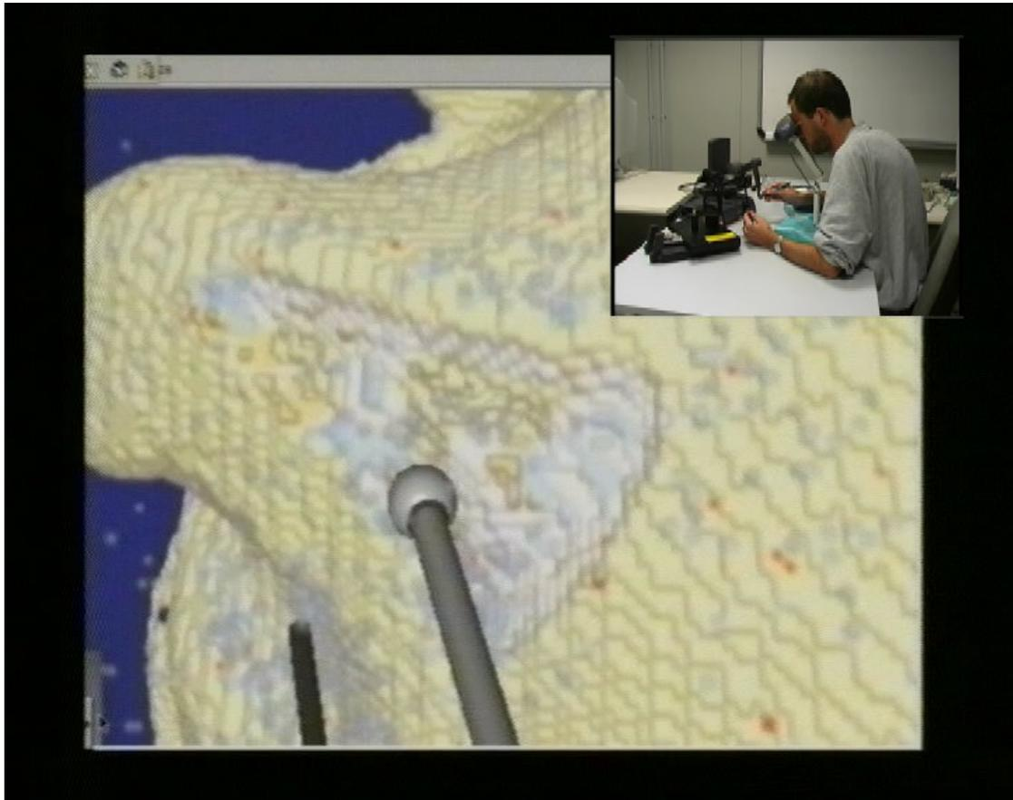
**Figure 3: Snapshot from a video demonstration of a simulated mastoidectomy. The central image show the image viewed by the training surgeon with bone, water, blood and manipulators. In the top right corner it is possible to see the corresponding external view with the training surgeon feeling the haptic feedback through the Phantoms while observing the scene in the binocular display**
