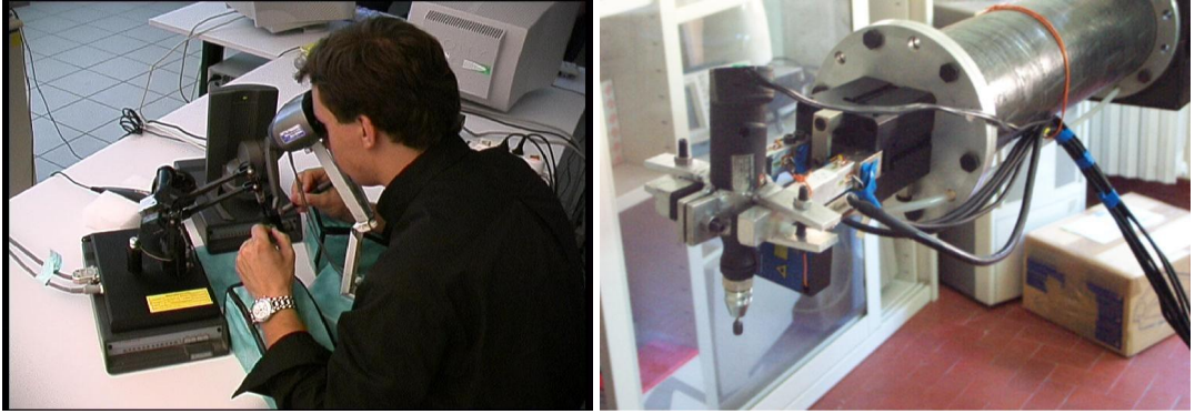
Figure 1: Surgical simulator setup vs experimental setup : on the left the virtual surgical training system user interface is composed by two phantom devices that provide force feedback for sucker and burr, as well as an N-vision binocular display that presents images to the user; on the right the experimental setup for measuring contact forces between the burr bit and the bone
