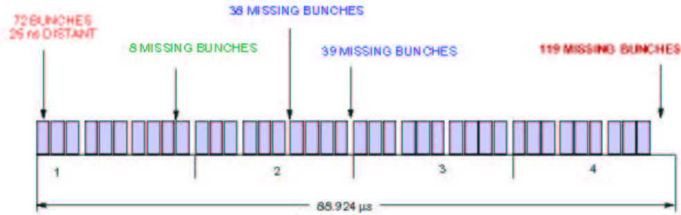
Figure 2.4: Bunch disposition inside the LHC
