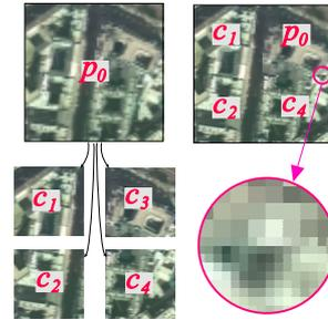
**Figure 8:** On the left side an example of a node with its four children (top-view). In the right side the representation used when only nodes  $c_1$ ,  $c_2$  and  $c_3$  can be locked, with a zoomed image of the border region between the two resolutions.
