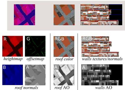
**Figure 2:** Improved version of BlockMap data structure.
