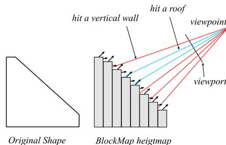
**Figure 3:** Left: original shape. Right: BlockMap encoding. The corresponding tiles are marked as roof, so also when the ray hits on the side, the roof data (normal, color, ambient occlusion) are used.
