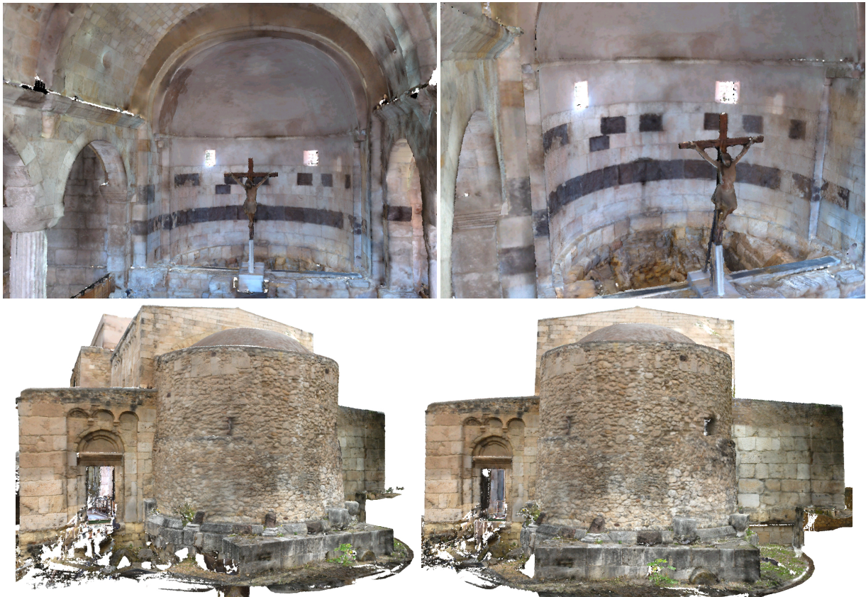
Fig. 9. Colored model of a church. A 72 million points 3D model of a church with color coming from a 1.6 Gpixel dataset (162 photos).
