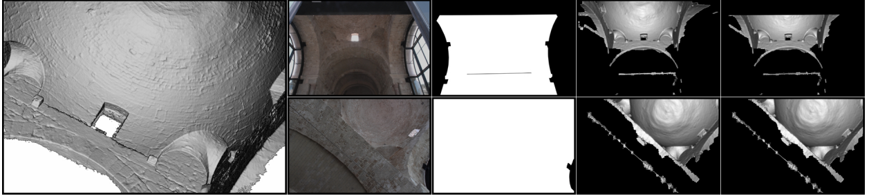
Fig. 3. Weighting Function Computation. From left to right: rendered point cloud; photos being blended; user defined stencil masks; per-pixel weights; masked per-pixel weights.
