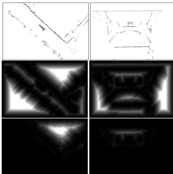
**Figure 5: Smooth weight generation.** Rows from top to bottom: edge map; distance transform; per-pixel weight modulated with distance transform term. Figures are modified in brightness and contrast in order to enhance readability.
