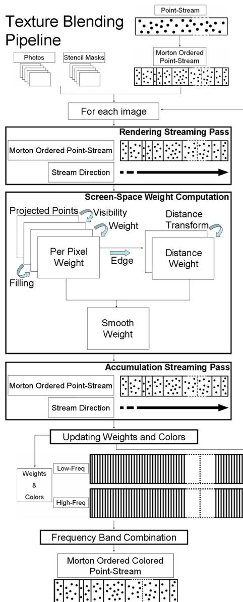
**Figure 1: Algorithm Pipeline.** The inputs are a point stream and an image set. After a fast pre-processing, for each image we render and fill in the point cloud, compute a per-pixel weight, and accumulate color, updating temporary out-of-core arrays for each frequency band. In the last streaming pass, we combine band contributions.
