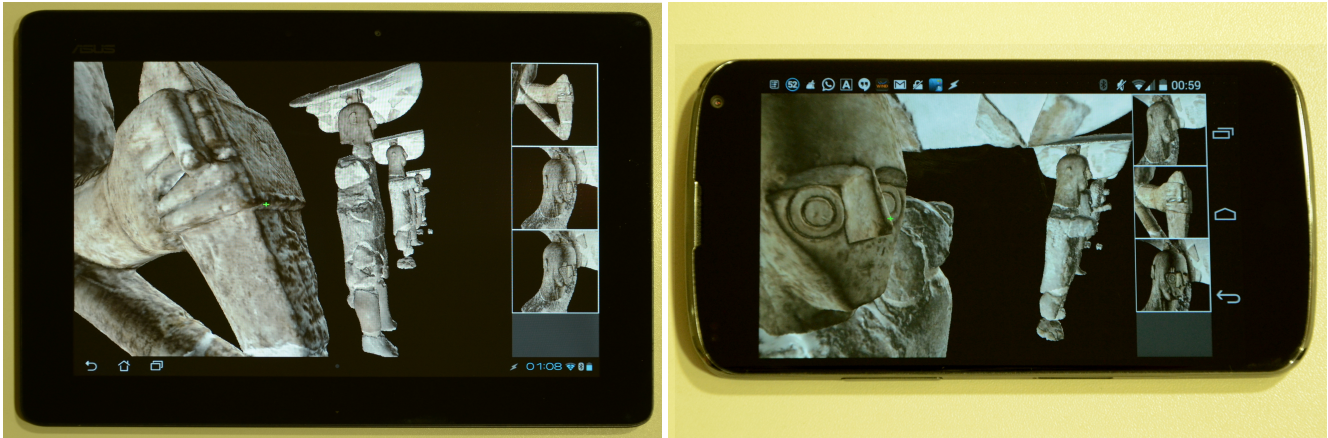
Figure 1: Remote virtual exploration of a scene composed by several high resolution statues on a Asus TF201 tablet (left image), and on a LG Nexus 4 smartphone (right image). During interaction, models are adaptively downloaded from the network, and knowledge of the currently rendered scene is exploited to automatically center a rotation pivot for the camera controller and to propose context-dependent precomputed viewpoints.
