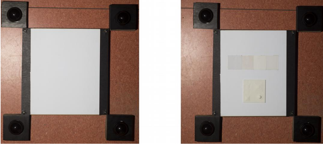
Figure 1: Left: Empty acquisition setup with white surface and four reflective spheres. Right: Setup with example objects (paper samples and 3D printed target)
