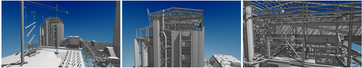
Figure 1: The PowerPlant scene voxelized to a 64K^3 resolution and stored as a Symmetry-aware Sparse Voxel DAG (SSVDAG). The total non-empty voxel count is nearly 6 billions, stored in less than 86MB at 0.123 bits/voxel. A sparse voxel octree would require 16.2GB without counting pointers, i.e. over 200 times more, while a Sparse Voxel DAG would require 167MB, i.e., nearly the double. Primary rays as well as hard shadow are raytraced directly in the SSVDAG structure, and shading normals are estimated in screen space.
