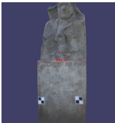
Figure 6. Measurement of distances in the point cloud of a statue.
