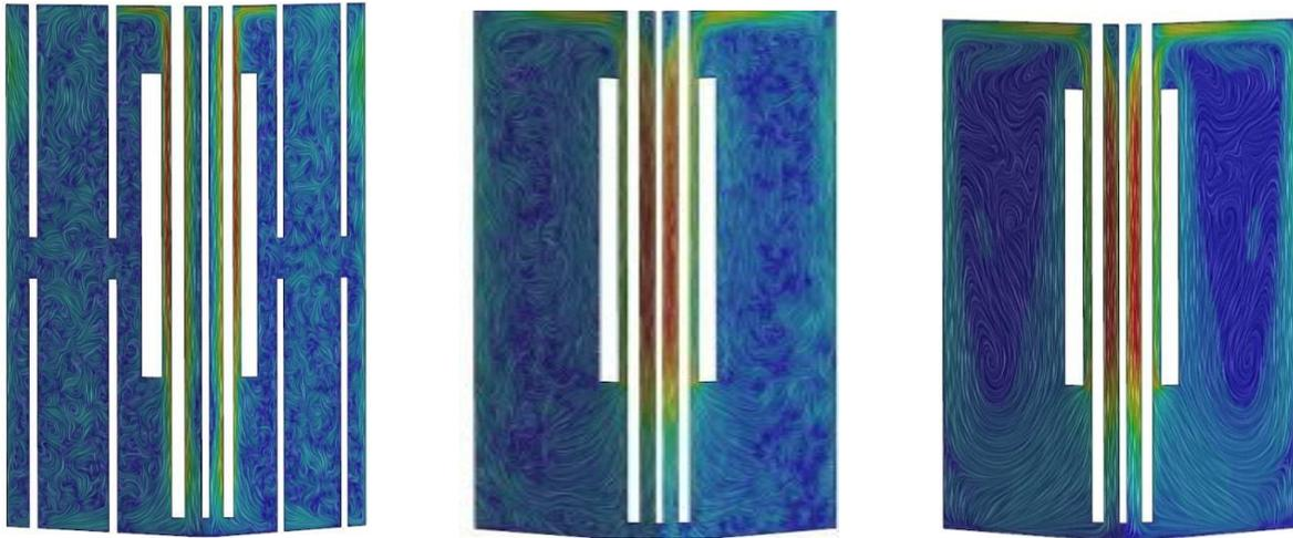
Fig. 17 Velocity vectors in SESAME –stand configuration (left) compared with the same configuration in a simplified geometry (center) and with the correct configuration of velocity field in simplified geometry (right)
