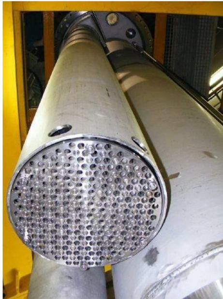
**Figure 4: View of the ICE HX installed into the test section.**
