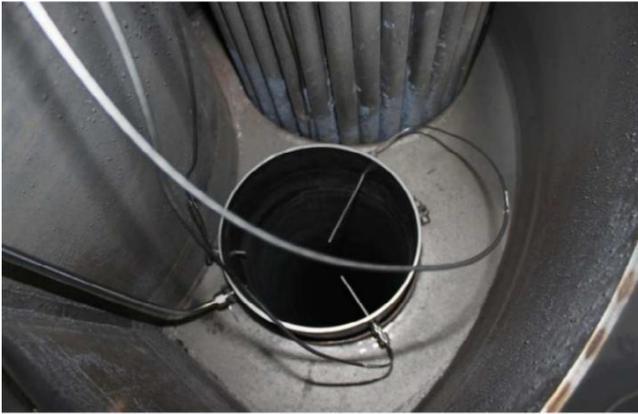
Figure 14: TCs installed at the riser exit
