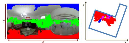
Figure 2: **Image segmentation and resulting facets.** Left: our super-pixels conservative segmentation. Right: the same ceiling and floor super-pixels represented as *facets* (see Sec. 3.2).
