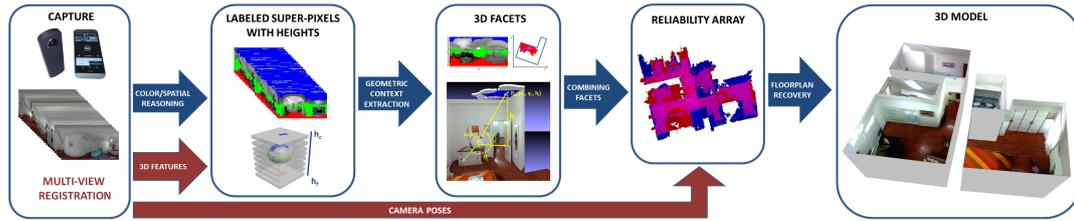
Figure 1: **Method pipeline.** Starting from few overlapping spherical images, we recover sparse 3D features and registered cameras. Such global information is used to enrich a per-image labeling into wall, ceiling and floor-superpixels, to robustly create 3D facets and segmentation reliability maps. A fusion approach finally generates a global 3D model.
