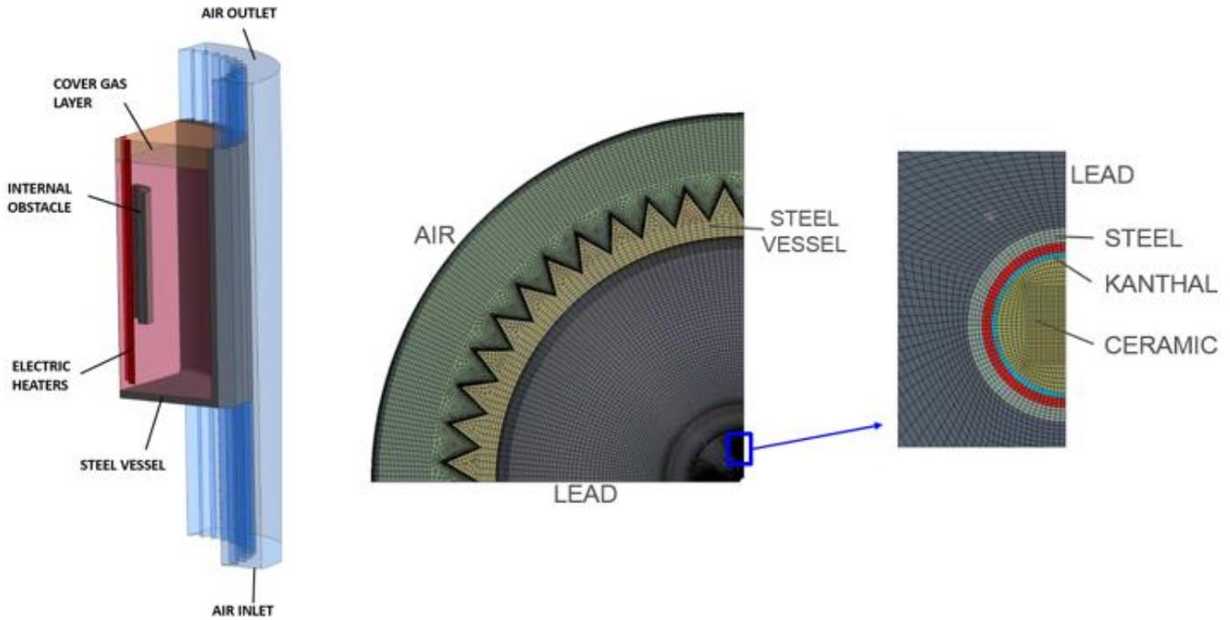
Figure 3: Computational geometry (left), computational mesh (right) of the CVR model
