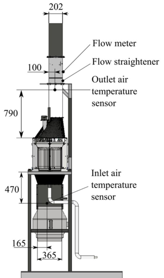
Figure 2: Layout of the air channel
