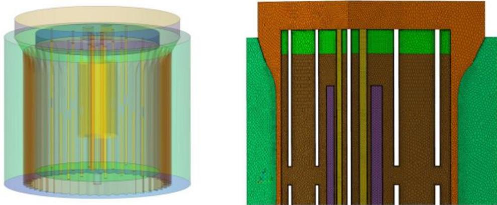
Figure 4: Computational geometry (left) and computational mesh (right) of the CRS4 model (Melichar 2018)
