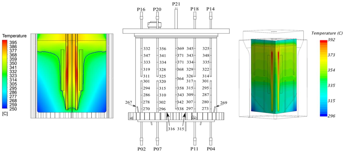
Figure 5: Results of CVR model (left), experimental data (middle) and CRS4 model for 4 kW heaters power and 0.101 kg/s air flow rate
