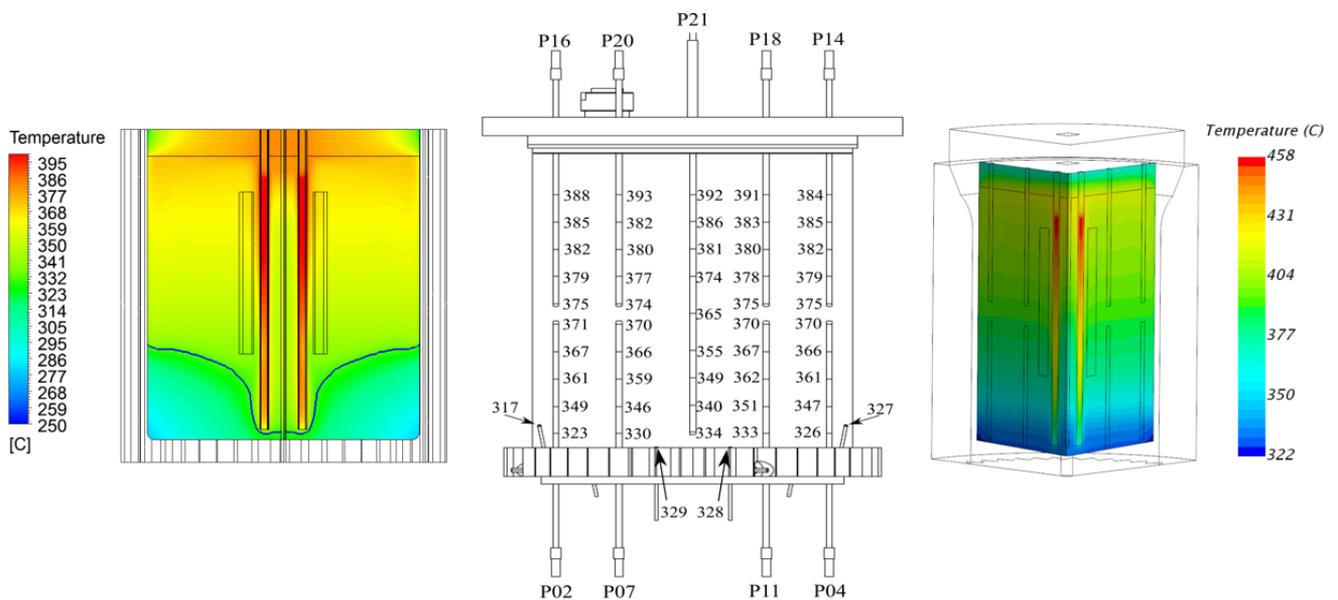
Figure 7: Results of CVR model (left), experimental data (middle) and CRS4 model for 5.6 kW heaters power and 0.145 kg/s air flow rate
