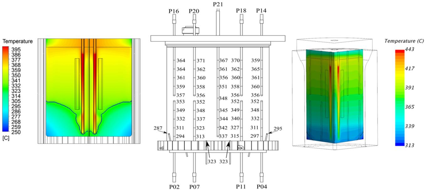
Figure 8: Results of CVR model (left), experimental data (middle) and CRS4 model for 5.6 kW heaters power and 0.167 kg/s air flow rate
