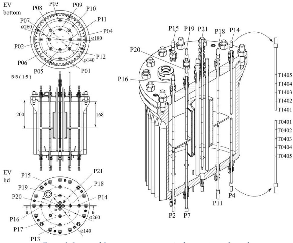
Figure 1: Layout of the temperature sensors in the experimental vessel
