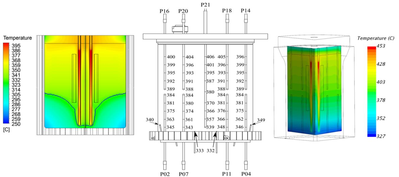
Figure 6: Results of CVR model (left), experimental data (middle) and CRS4 model for 4.96 kW heaters power and 0.101 kg/s air flow rate
