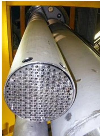
Figure 3: View of the ICE HX installed into the test section.
