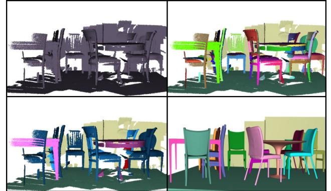
**Figure 14:** Data-driven object reconstruction. The search-classify approach [NXS12] initially over-segments the scene (top-right) and search-classifies meaningful objects in the scene (bottom-left); these are reconstructed by templates (bottom-right) overcoming the high clutter present in the input scans (top-left). Source images courtesy of Nan et al. [NXS12].
