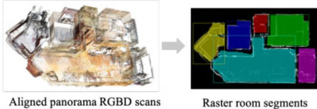
**Figure 3: Room segmentation from aligned RGB-D scans.** Aligned panorama RGB-D images are turned into a floorplan graph starting from room segments (raster) from a top-down projection image, consisting of point density and mean surface normal. [CLWF19]
