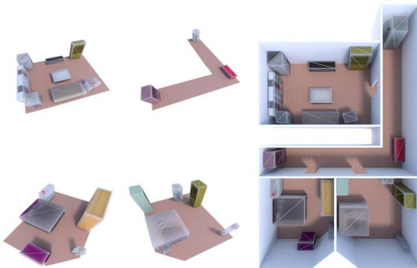
**Figure 13:** Clutter models using virtual plane-sweep reconstruction. The E2P transform [PPG<sup>\*</sup>18] is applied locally for each single object segmentation and then merged in a plane-sweep fashion. Virtual plane-sweep camera is assumed to be a top-down view [PGJG19].
