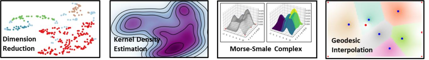
Fig. 2. **Density-based automatic transfer function:** The computation pipeline (left to right) starts by attribute projection through dimensionality reduction, density-function computation through kernel density estimation, generating Morse-Smale complex manifolds, and finally performing the geodesic interpolation.
