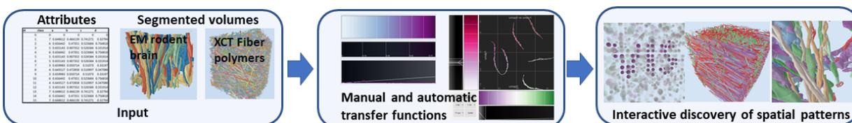
Fig. 1. Inspired by word search puzzles, we present *Volume Puzzle*, a framework that allows us to interactively and/or automatically reveal spatial patterns from segmented volumes with associated multivariate attributes
