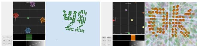
Fig. 4. **Visual analysis of synthetic data:** two examples of test volumes containing spheres associated with scalar attributes. Only The automatic transfer function is able to highlight the spatial pattern.
