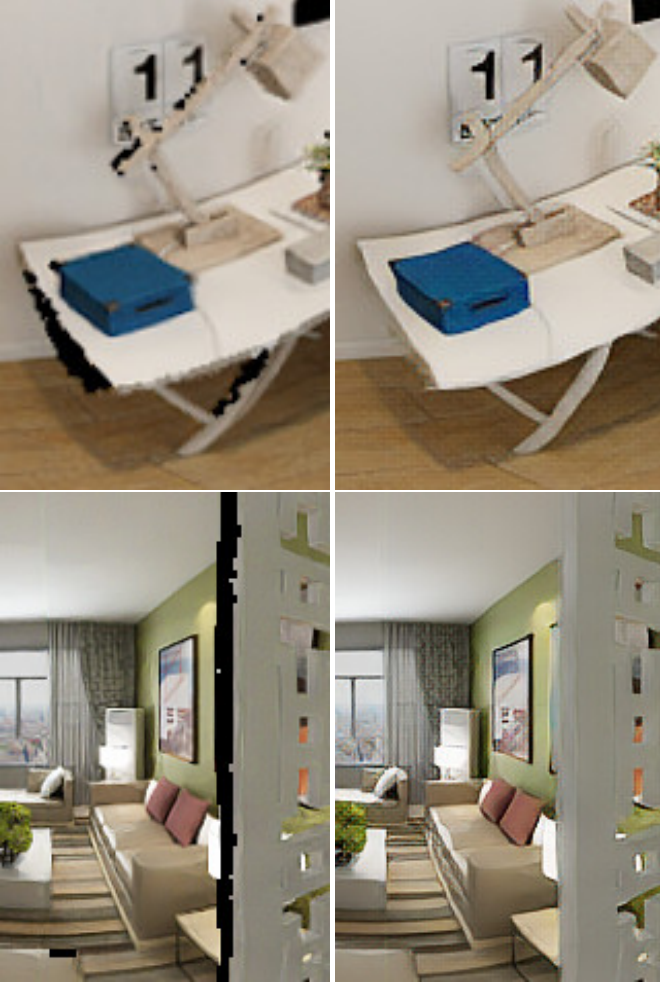
Fig. 6: Reprojected vs. synthesized image Two examples from different scenes. On the left, we see a detail of a reprojected image slice, where disoccluded areas are apparent. On the right, we see the output of the view synthesis network.
